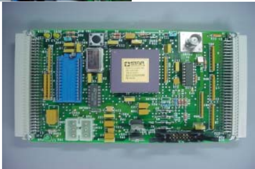
Digital Signal Processor unit. Used to analyze and trigger on energy burst as it entered system.
