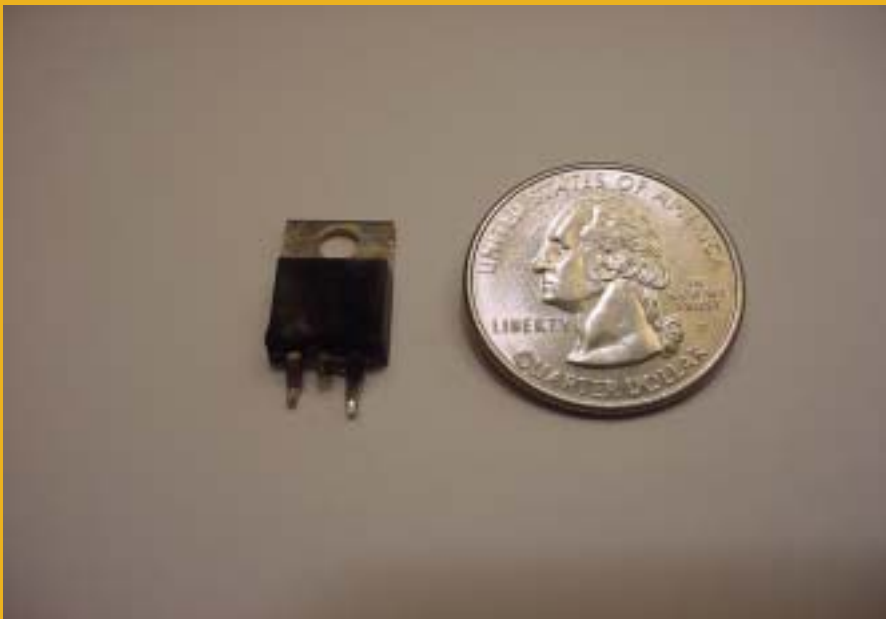
View of burned Field Effect Transistor (FET) commonly used in DC to DC converter power supplies.
